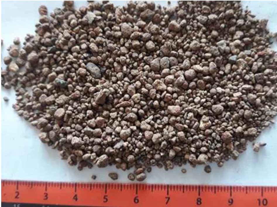
Fig.2 Sorbent Halosorb after 7 years of operation
